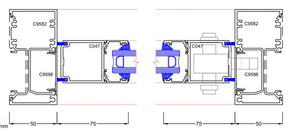
Pivot door frames are better manufactured from Centre Glaze framing where the flush filler is centrallised on the frame.
